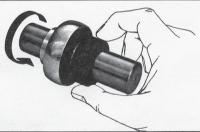
4. With drift pin in collar hole, strike in direction of shaft rotation to lock.
